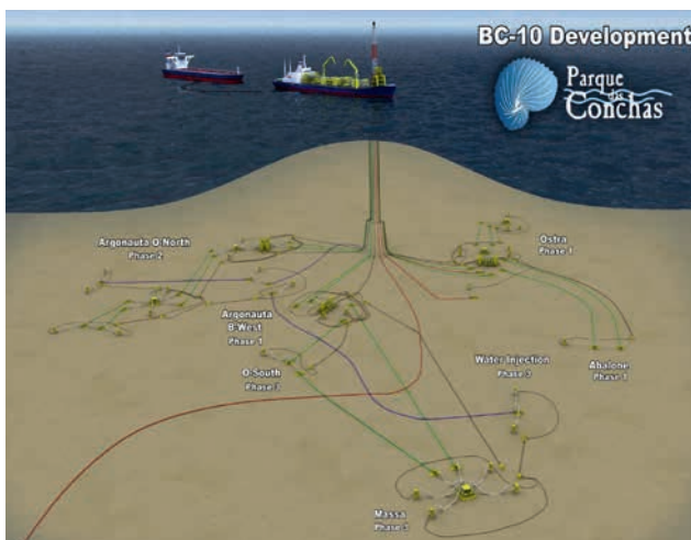
Figure 1 Schematic of the Parque das Conchas (BC-10) infrastructure showing the three phases of development and tie-back to the centrally located floating production, storage and offloading (FPSO) vessel, the Espírito Santo .
