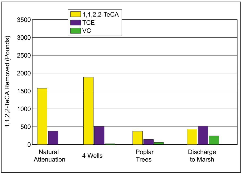
Figure 6. Simulated Mass Removal by Integrated Remedial System
