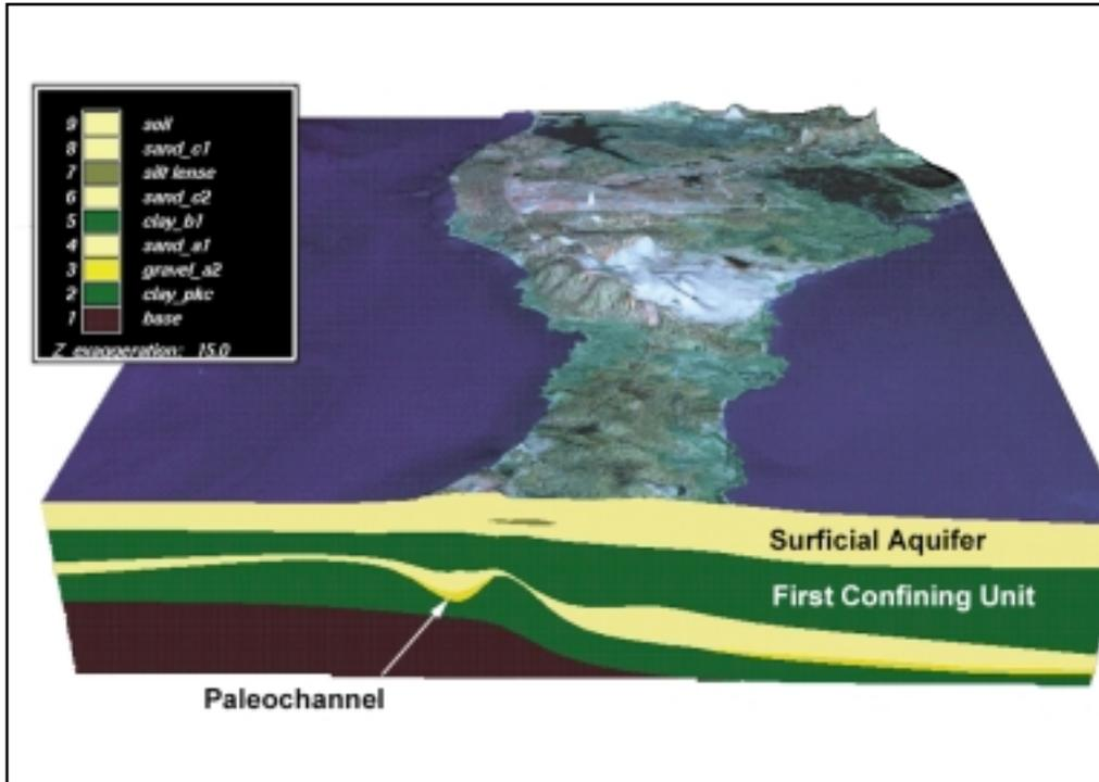
Figure 3. 3-D Geospatial Model Illustrating the Hydrostratigraphic Units
