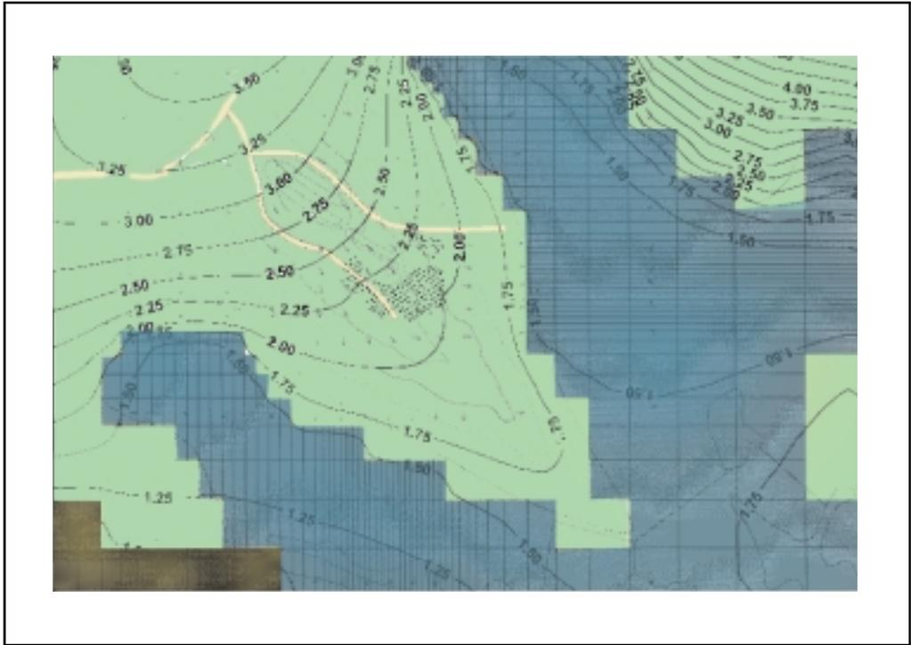
Figure 5. MODFLOW Grid Showing Simulated Hydraulic Head
