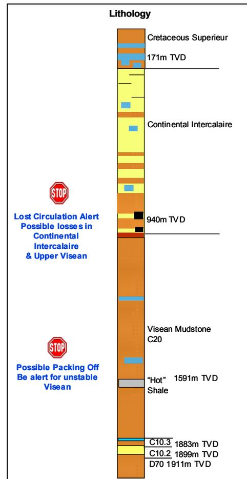
Fig. 3: Krechba field lithology column and drilling hazards
