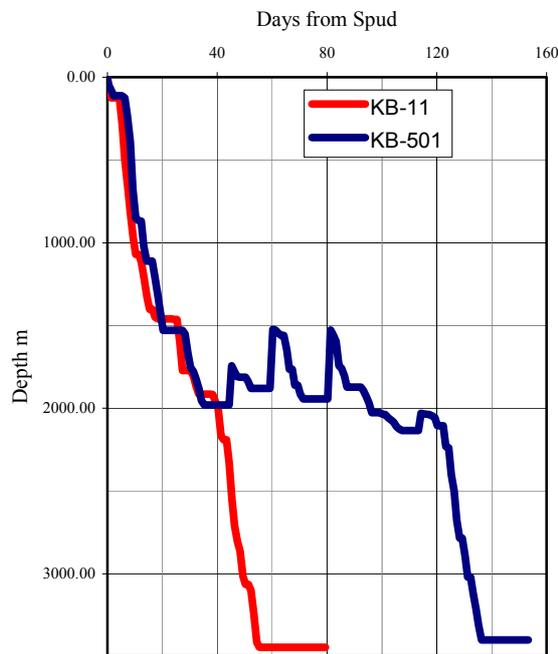
Fig. 5: Comparison of KB-501 and KB11 time vs. depth plots
