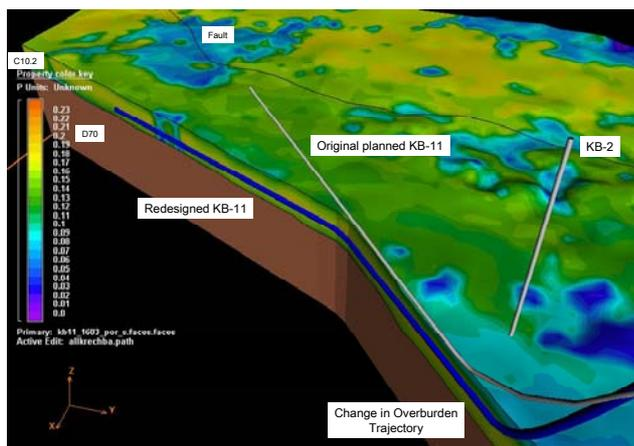
Fig. 4 – KB-11 original and revised directional plan
