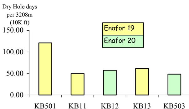
Fig. 8: Krechba drilling progress learning curve
