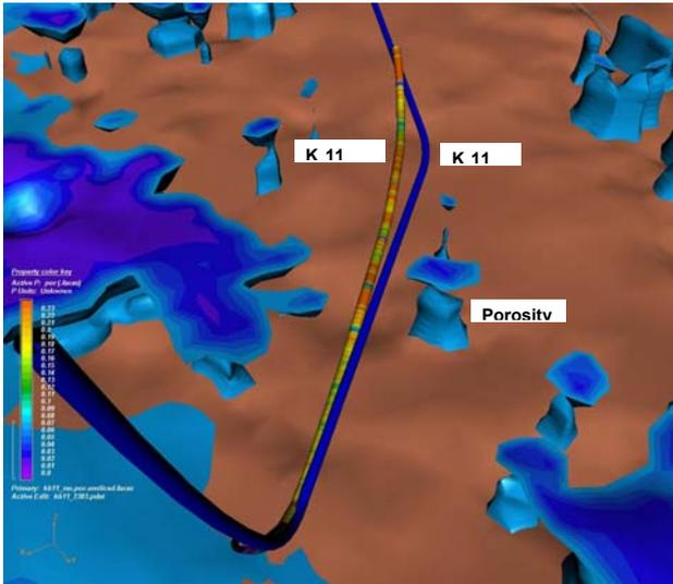
Fig. 6: KB-11 area showing porosity < 7%, planned well in blue and partially drilled well colour coded with real time porosity 766m into reservoir section
