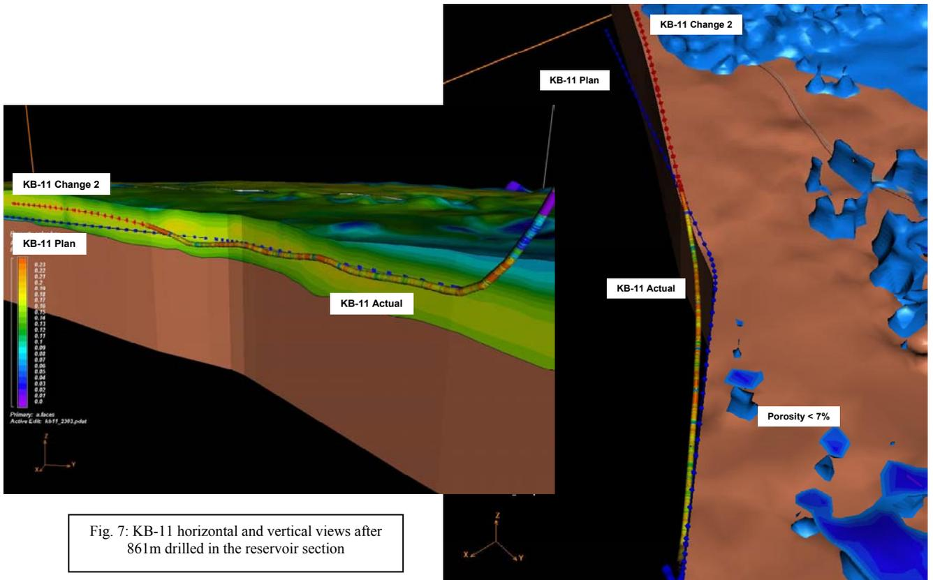
Fig. 7: KB-11 horizontal and vertical views after 861m drilled in the reservoir section
